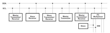
Figure 6.3 System Configuration
