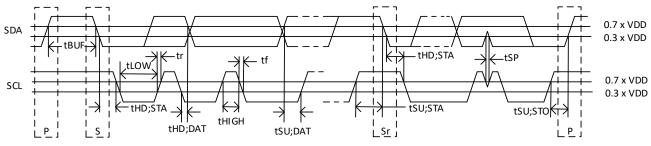
Figure 5.1 Definition of timing on I<sup>2</sup>C-bus
