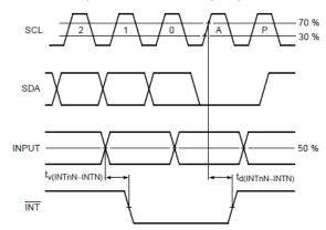
Figure 5.4 Expanded view of read input port register
