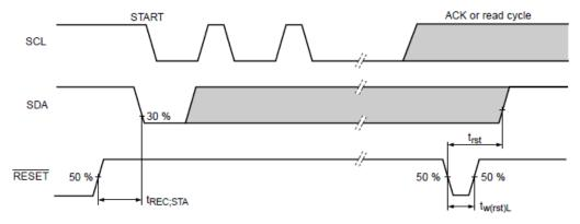
Figure 5.2 Definition of RESET timing
