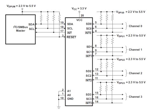
Figure 7.1 Typical Application Schematic
