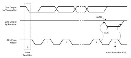
Figure 6.4 Acknowledgment on the I<sup>2</sup>C Bus
