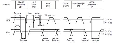
Figure 5.3 I<sup>2</sup>C-bus timing diagram
